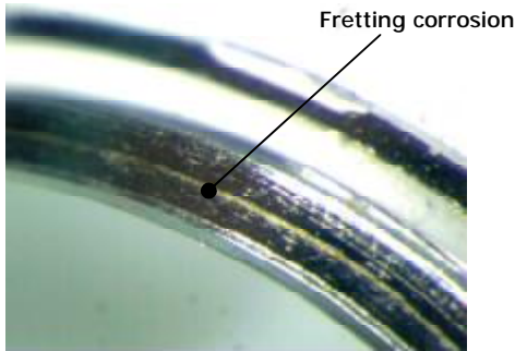
Fig. 5: Photo of an outer race (20AP) of standard bearing
