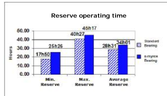
Fig. 13: Table comparing the results of the wear test
