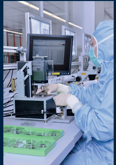
Bench for torque measurement of a pumping unit
