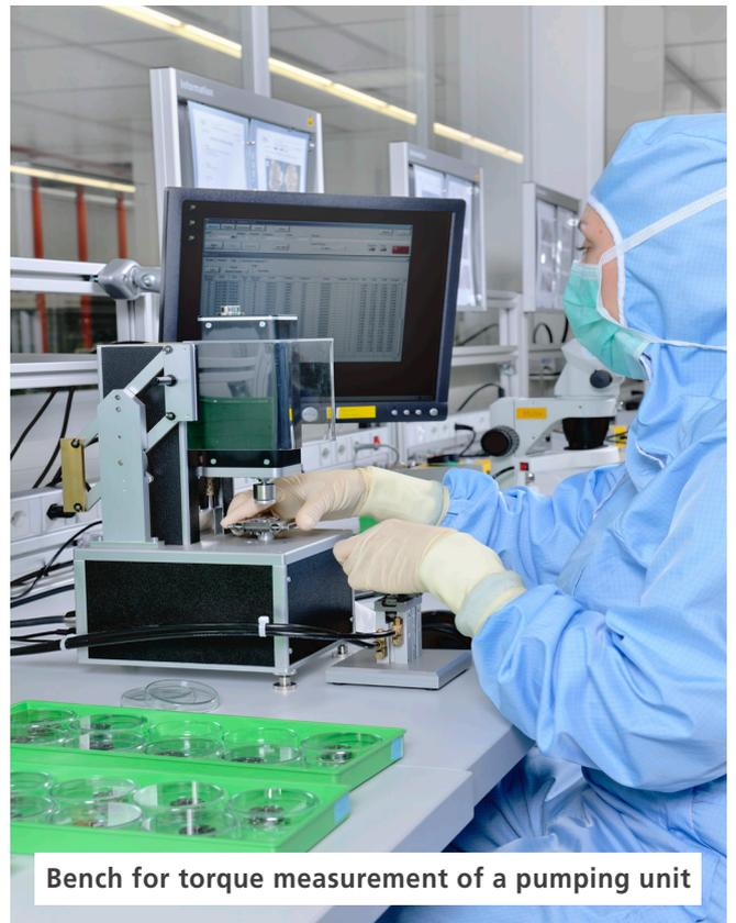
Bench for torque measurement of a pumping unit
